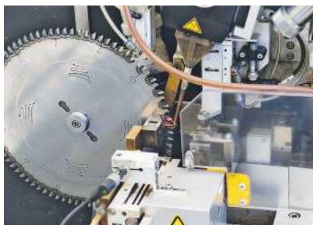
Each tip is induction heated to form a solid bond to the blade
